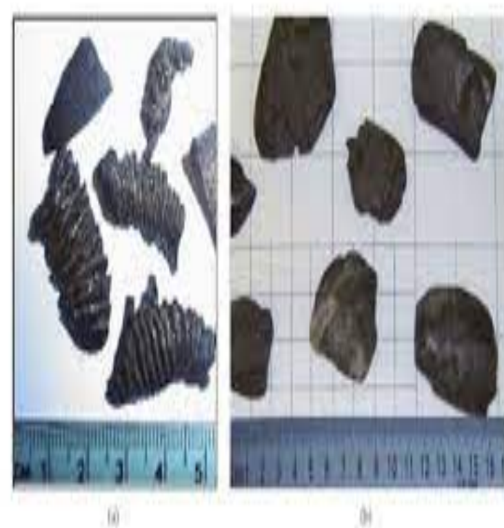
FIGURE 8. Drilling cuttings. (a) Normal PDC cuttings of shales; (b) blocky cuttings from a formation with preexisting fractures.
